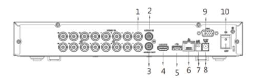
VIDEO IN Network Interface 1 6 2 AUDIO IN, RCA Connector RS485 Interface AUDIO OUT, RCA Connector DC 12V Power Input 3 **HDMI Interface** VGA Interface 4 9 USB Interface Power Switch 5
